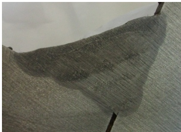
GMA welding sample, weld with the new AMT control concept under 5 bar pressure!
