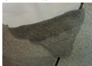
GMA welding sample, weld with the new AMT control concept under 5 bar pressure!
