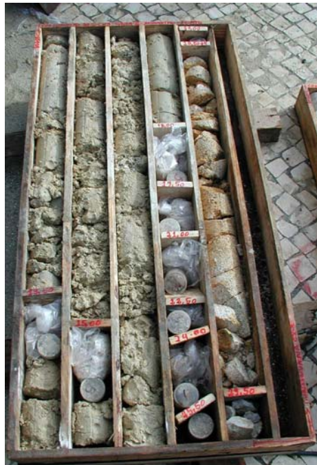
Figure 7: Core samples of heterogene geology
