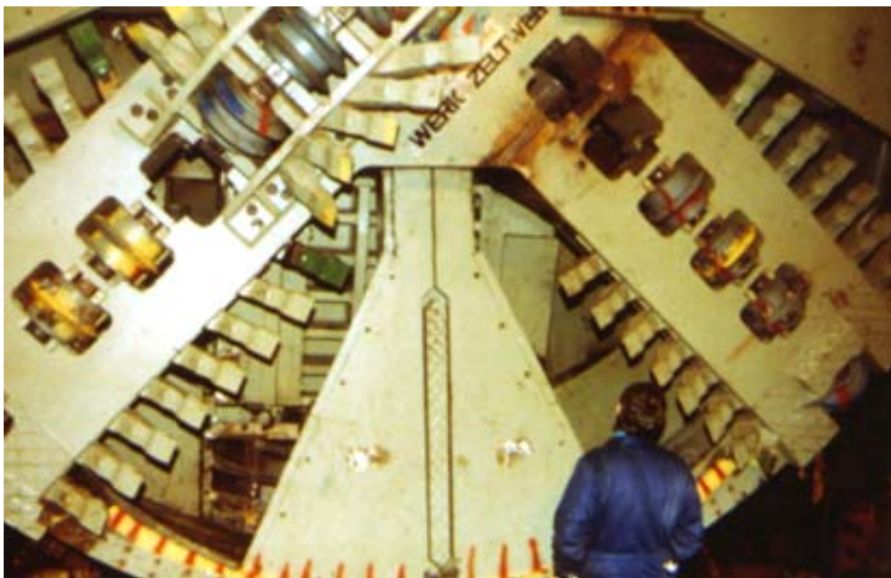
Figure 14: Tool combination – discs and scrapers
