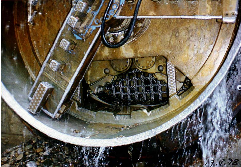
Figure 17: Inlet of transportation pipe line with grill and crusher
